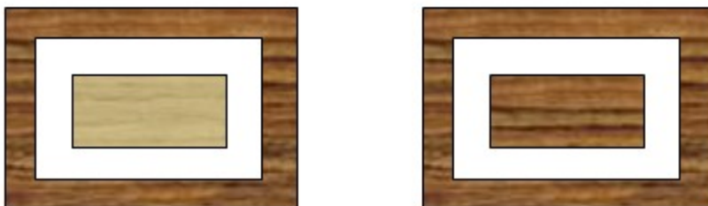
Fig. 1 A packaging with a white frame and a transparent "window" on a wooden surface. Left: previous behavior with the paper tint printed on transparent area. Right: only the white frame is printed with the paper tint, the transparent area is clear.
