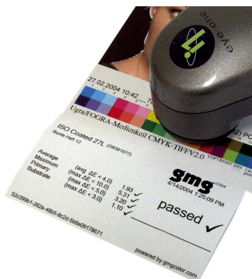
Fig. 1 Control Strip and Label verifying that the measured values are within the tolerances defined in the standard.
